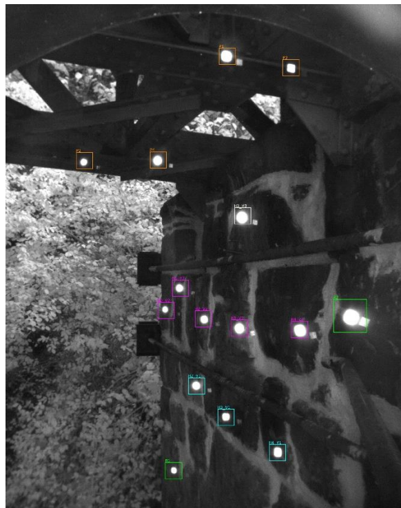
Left: View of the historical railway bridge with the solar power supply and one of the AIMsight autonomous optical monitoring systems. Right: View of the abutment wall monitored by the AIMsight system
