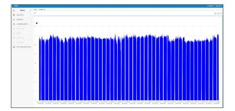
This WMS screenshot shows the histogram with the maximum displacement for each train passage. In the plot periods without data correspond to the night train stops. Enlarging the zoom makes possible to verify at which time the train pass on the FLX-Rail® installation point, as well as the corresponding maximal vertical displacement reading.
